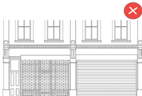
Picture 37. External Roller shutters are not appropriate.
