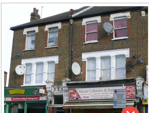
Satellite dishes shouldn't usually be mounted on the front of buildings
